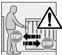
All persons using the gate system must be shown how to operate it properly and safely. Demonstrate and test the mechanical release as well as the safety return. To do this, halt the closing gate by grasping it with both hands. The gate system should gently cut out and initiate the safety return. The same should happen during the opening cycle, i.e. the gate system should gently cut out and initiate the safety return.
