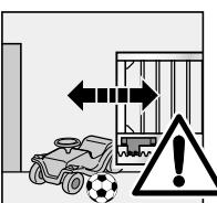
Permanently installed controls (such as buttons or similar devices) should be installed within sight of the gate but well away from any moving parts and at a height of at least 1.5 metres.
