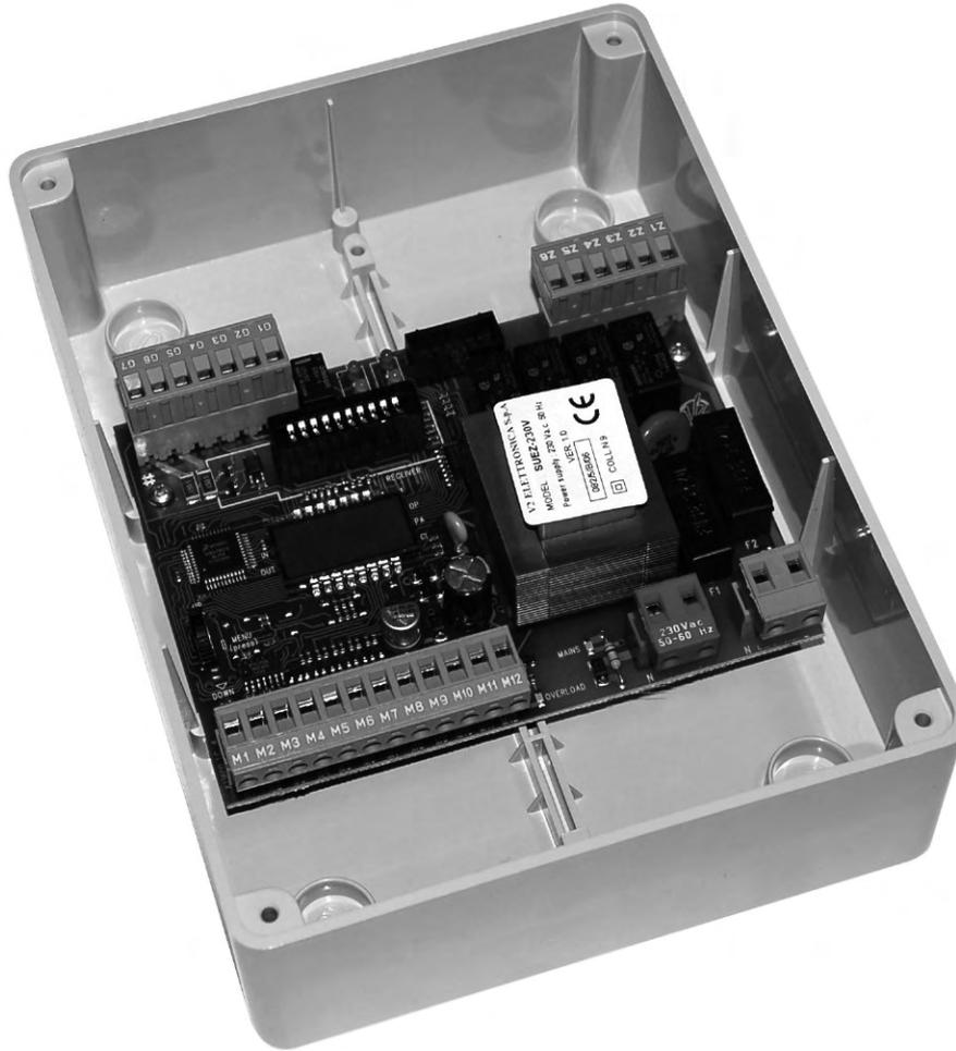
**I** CENTRALE DIGITALE PER IL CONTROLLO DELLE LAMPAD E SEMAFORICHE
