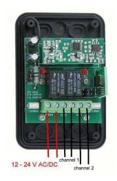
This new receiver has an important advantage compared to the previous models, since it allows us to have up to 4 receivers in the same device, just by changing the jumpers' position.
