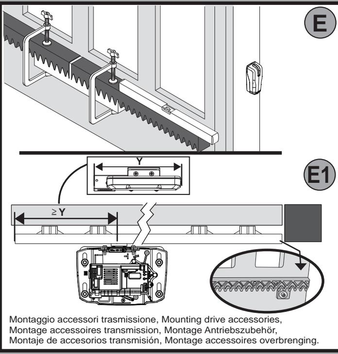
Montaggio accessori trasmissione, Mounting drive accessories,
