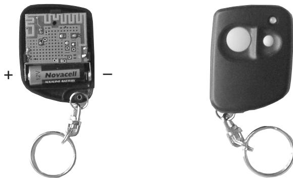
Every hand transmitter has its own security code, which can be programmed into the drive.
